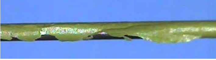
Loss of PFOA-free PTFE adhesion on guidewire after being soaked in a 0.9% saline solution at 80°F for 30 minutes.
