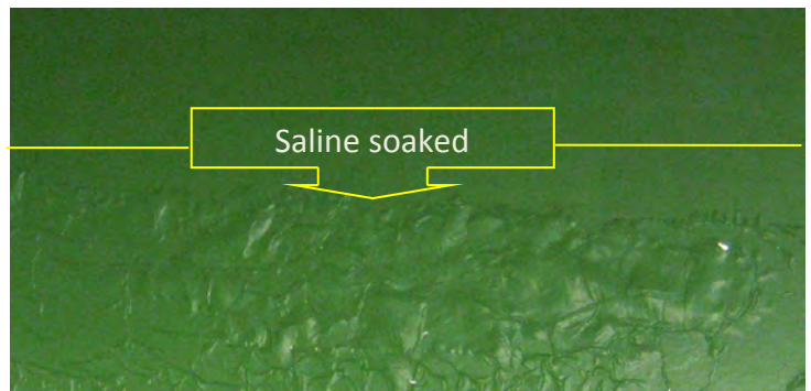
What appears to be a smooth, bonded no-PFOA PTFE coating on this panel, once immersed in saline for 30 minutes at 80 Fahrenheit, starts to delaminate otherwise stainless steel panel.
