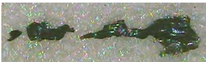
Using the high-tack tape employed in the FluoroBond® process, flakes of commercially available PFOA-free PTFE coating are pulled off easily from a guidewire that has not been treated with the FluoroBond® process. (100 X)
