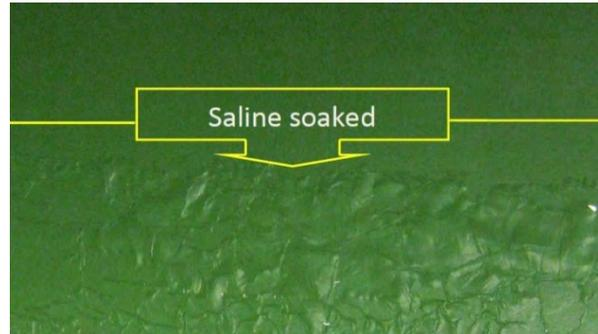
Figure 1—Effect of saline immersion on PTFE coated test panel.
